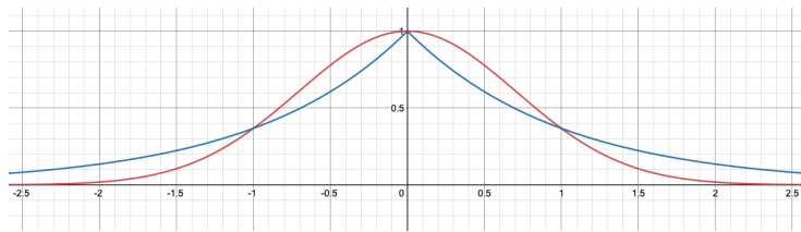
Figure 10.2: The red curve is a zero-mean Gaussian PDF and the blue curve is a zero-mean Laplace PDF for the weight w \in \mathbb{R} .
